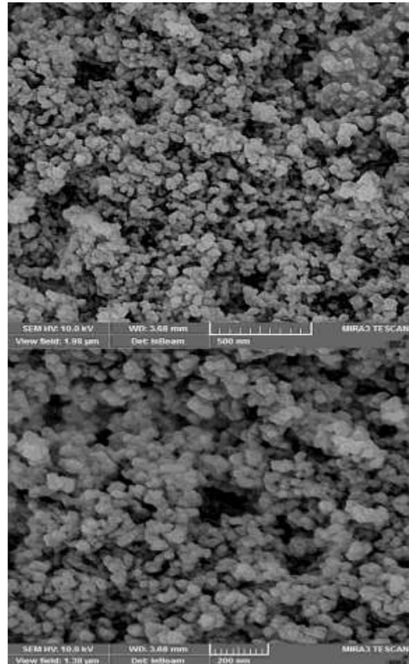
Fig. II. SEM images of Zinc oxide nanoparticles
