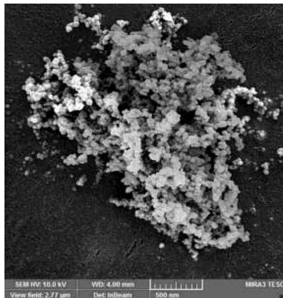
Fig 1. SEM image of Iron oxide nanoparticles
