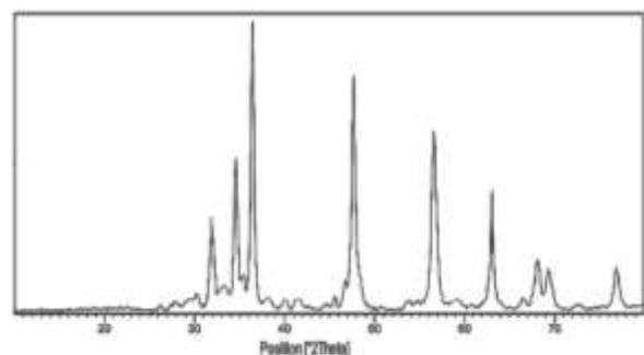
Fig.III. XRD pattern of zinc oxide nanoparticles
