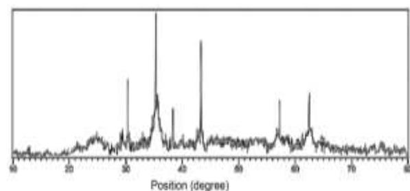
Fig. IV. XRD pattern of iron oxide nanoparticles
