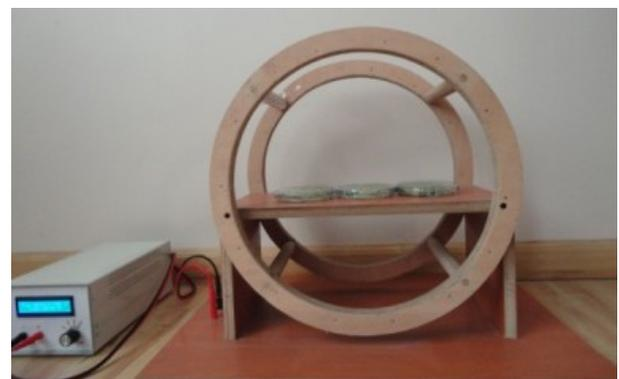
Fig. 1. Electromagnetic field exposure arrangement
