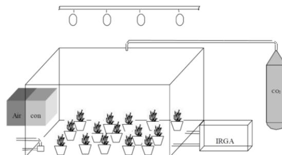
Fig. V. Set-up of the labeling chamber for isotopic labeling of whole plants (Sanchez et al, 2000)
