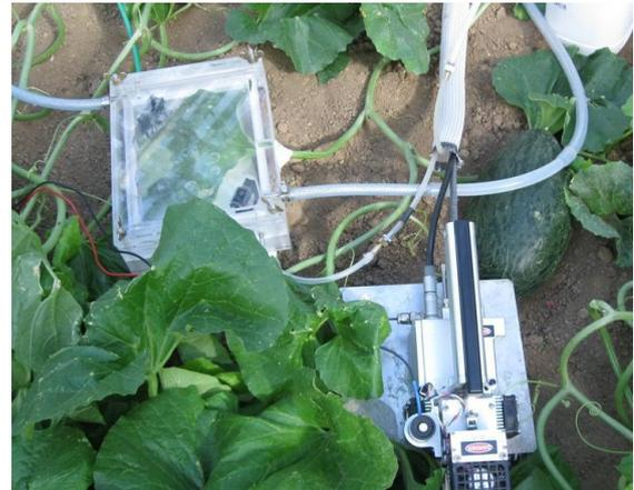
Fig. I. Labeling chamber coupled to the Licor-6400 gas exchange system (Barzegar, 2011).
