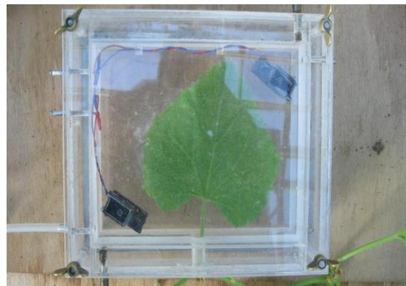
Fig. II. Single leaf labeling chamber with approximately 350 cm<sup>2</sup> size (Barzegar, 2011).
