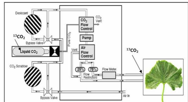
Fig. III. LI-6400 open system of photosynthetic gas exchange (IRGA); the incoming air stream can be conditioned for  $\text{CO}_2$  concentration, humidity, and temperature. There are chemical tubes for scrubbing  $\text{CO}_2$  and  $\text{H}_2\text{O}$ . The air was diverted through these tubes and  $^{12}\text{CO}_2$  from the incoming air was removed, and  $^{13}\text{CO}_2$  source injected to system.
